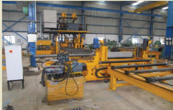
H-Beam Assembling with SAW
