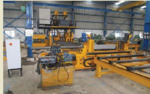
H-Beam Assembling with SAW
